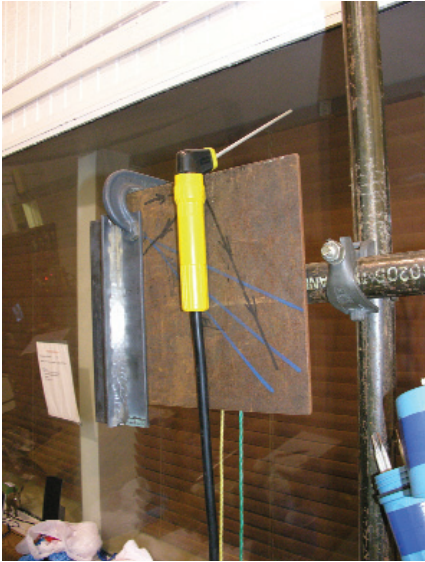
Fig. 5 — Underwater welding station setup.
